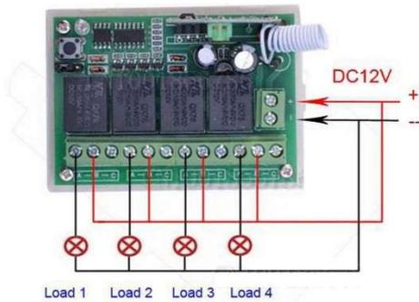
Control Electric Door Wiring Diagram
