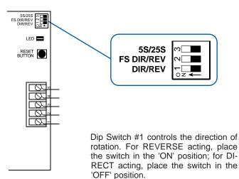
Dip Switch #2 determines the fail safe direction either clockwise or counterclockwise. The factory setting is in the 'OFF' position to 'fail' CCW to the 0° position. To 'fail' to the 90° position, place the switch in the 'ON' position.
