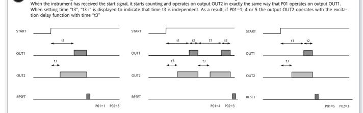
If OUT1 = 2 or 3, output OUT2 operates with the pass-band excitation function with time "t3":
