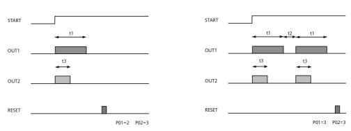
the start signal, it starts counting and operates on output OUT2 in exactly the same way that P01 operates on output OUT1. When setting time "t3", "t3 d" is displayed to indicate that time t3 is independent. if P01=2 or 3, output OUT2 operates with the pass-band excitation function with time "t1"-"t3": START START OUT1 OUT1 t3 . t3 **4**3 t3 OUT2 OUT2 OUT2 RESET RESET P01=1 P02=4 P01=5 P02=4
