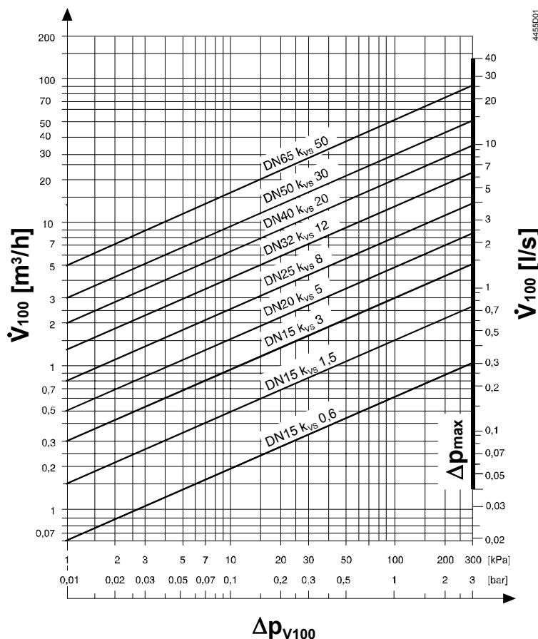
$\Delta p_{V100}$  = differential pressure across the fully open valve and the valve's control path A → AB by a volume flow  $\dot{V}_{100}$
