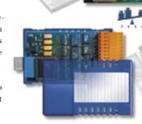
The Saia® PCD weighing module allows precise determining of weight or dosing with very different types of weighing or loading cells that are equipped with a resistance bridge. The signal from the cell is amplified, digitized and filtered in the weighing module, where it is then available to the user as a gross, tare or net weight •
