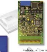
The four input channels of the temperature measurement module are electrically isolated from the PCD. To guarantee maximum flexibility in the application, each channel is fully configurable individually from software. For thermoelements types J and K, one can choose between internal or external compensation (CJC). For resistance temperature sensors (RTDs), a choice of sensor types is offered: Pt100 / Pt1000 / Ni100 / Ni1000 in optionally 2, 3 or 4-wire measurement technology.
