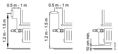
When mounted on poorly insulated outer walls, a thermally insulating layer should be fitted in between.
