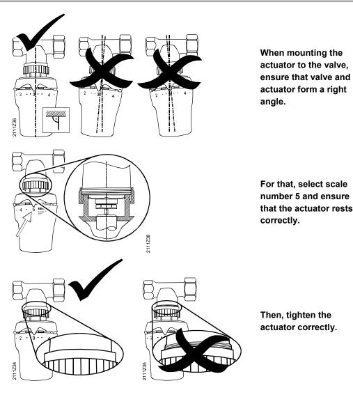
The sensing element of the thermostatic actuator must always be able to acquire the temperature of circulating room air.
