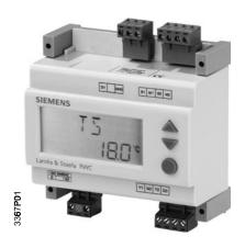
Fully autonomous, electronic temperature controller with P or PI response. Two temperature inputs for LG Ni 1000  $\Omega$  temperature sensors. One digital input for summer/winter or day/night changeover. Two modulating outputs with DC 0...10 V signal output, direct or indirect action. Entering or changing of all data via operating buttons on the controller, possible without additional tools.
