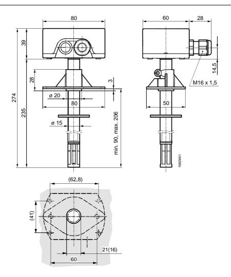
Drilling template with (without) mounting flange
