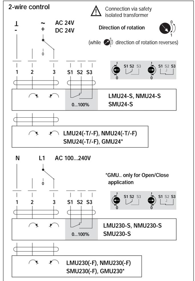
Wiring diagram: Modulating actuators—Parallel connection possible, please note the performance data.
